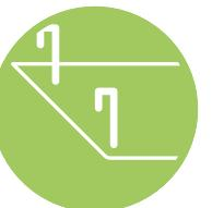
Secure the perimeter using 16 cm long nails at a distance of 30-50 cm between them.
