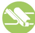
For **small surfaces** it is recommended to use adhesive tape. Lift and fold back both pieces of artificial grass. Place the adhesive tape between them and stick down the two pieces of artificial grass pressing firmly down.
