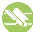
For **large surfaces** use two-component glue and joint tape. Lift and fold back both pieces of artificial grass. Place the joint tape between the two rolls (shiny side down). Apply the glue evenly across the tape and stick down the two pieces of artificial grass pressing firmly down.
